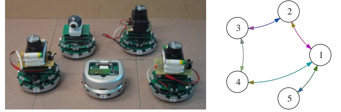
Fig. 1. Left: picture of the five Khepera III robots used in the experiment. Right: the undirected communication topology of the experiment.
