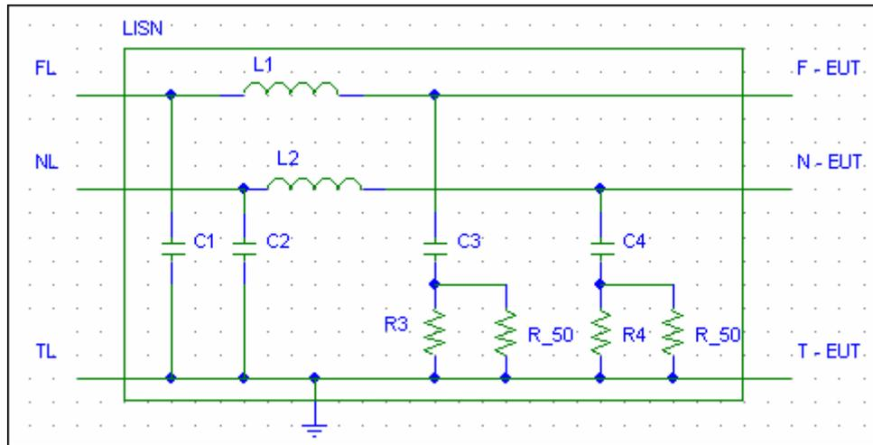
$$C_1 = C_2 = 1 \mu\text{F},$$
