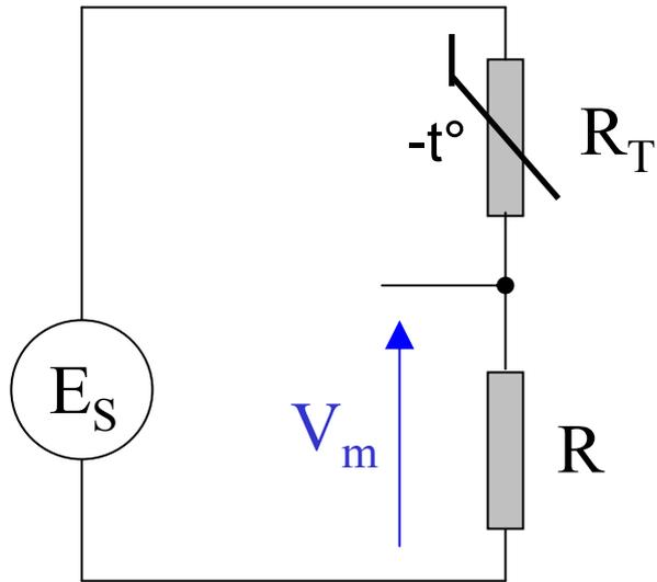
$$R_T = R_0 \exp \left\{ \beta \left( \frac{1}{T} - \frac{1}{T_{25^\circ C}} \right) \right\} = R_0 f(T)$$
