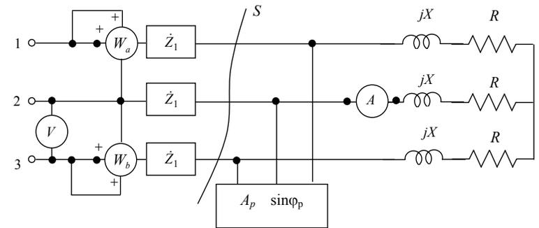
**Dati:**  $\dot{Z}_1 = 2 + 1j \Omega$ ,  $R = 1 k\Omega$ ,  $X = 2 k\Omega$ ,  $A_p = 12 kVA$ ,  $\sin \varphi_p = 0.707$ ,  $f = 50 Hz$ .
