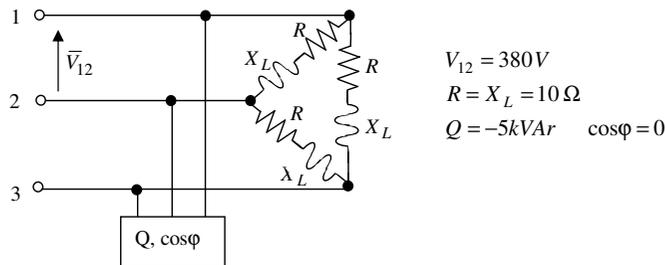
Risultato: a)  $\dot{A} = 21.66 \text{ kW} + j16.66 \text{ kVAr}$ , b)  $C_{\Delta} = 45.33 \mu\text{F}$ .
