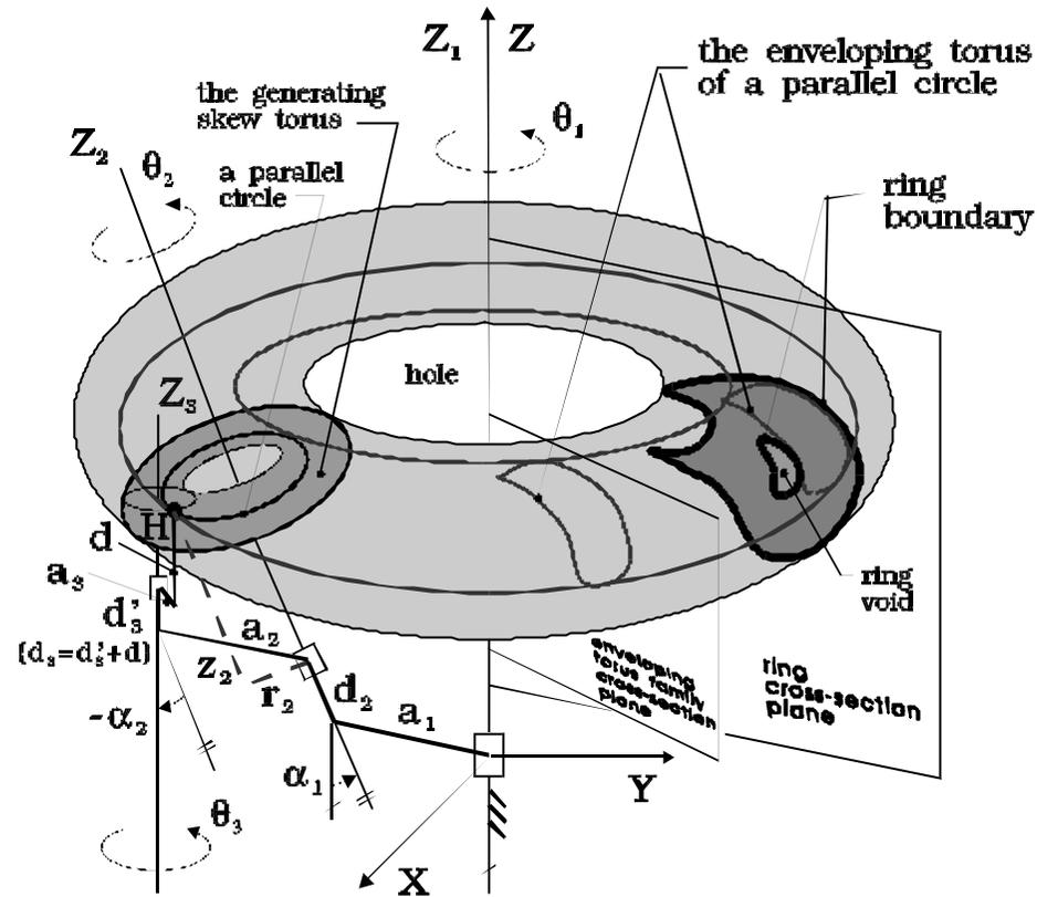
Fig.2 Design parameters and workspace geometry for 3R manipulators.
