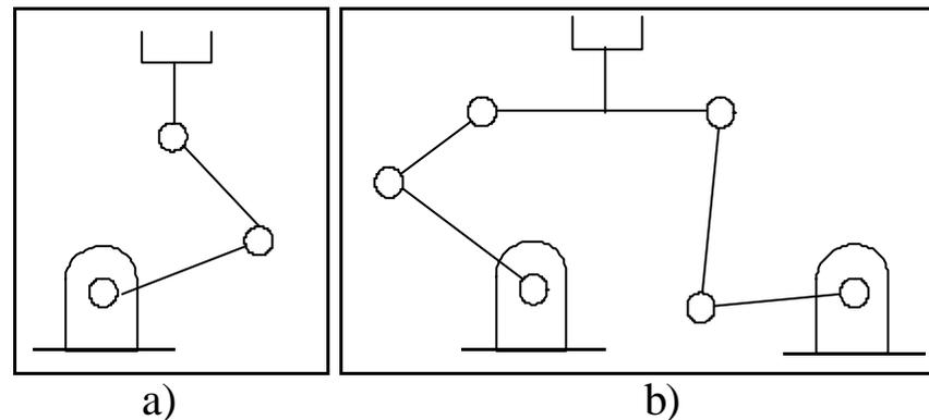
*Fig.3.2: Planar examples of kinematic chains of manipulators: a) serial chain as open type; b) parallel chain as closed type.*
