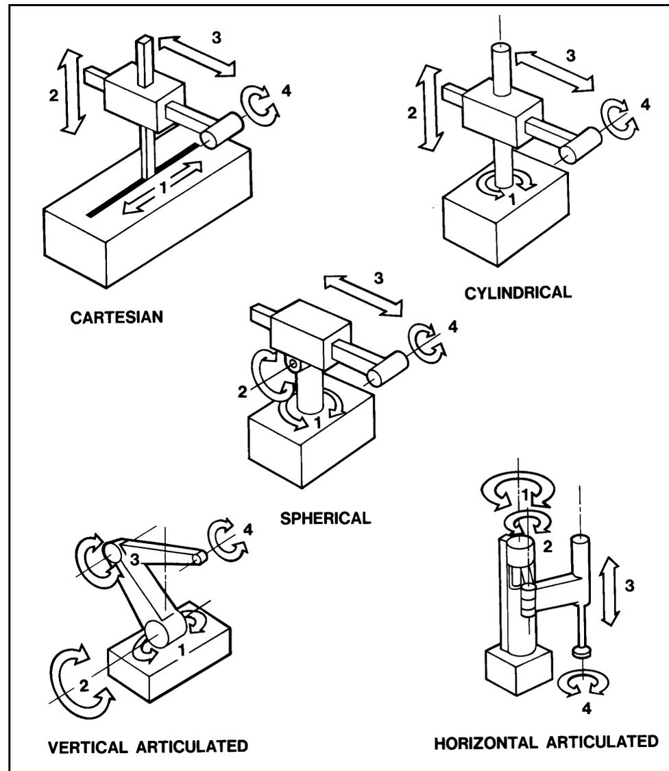
*Fig.3.4: Manipulator architectures for industrial robots.*
