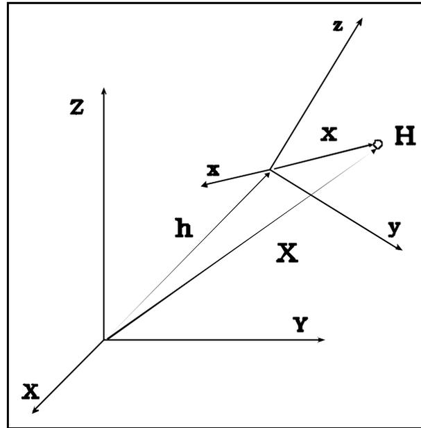
Fig.3.7: Vectors for relative position and orientation between two reference frames.
