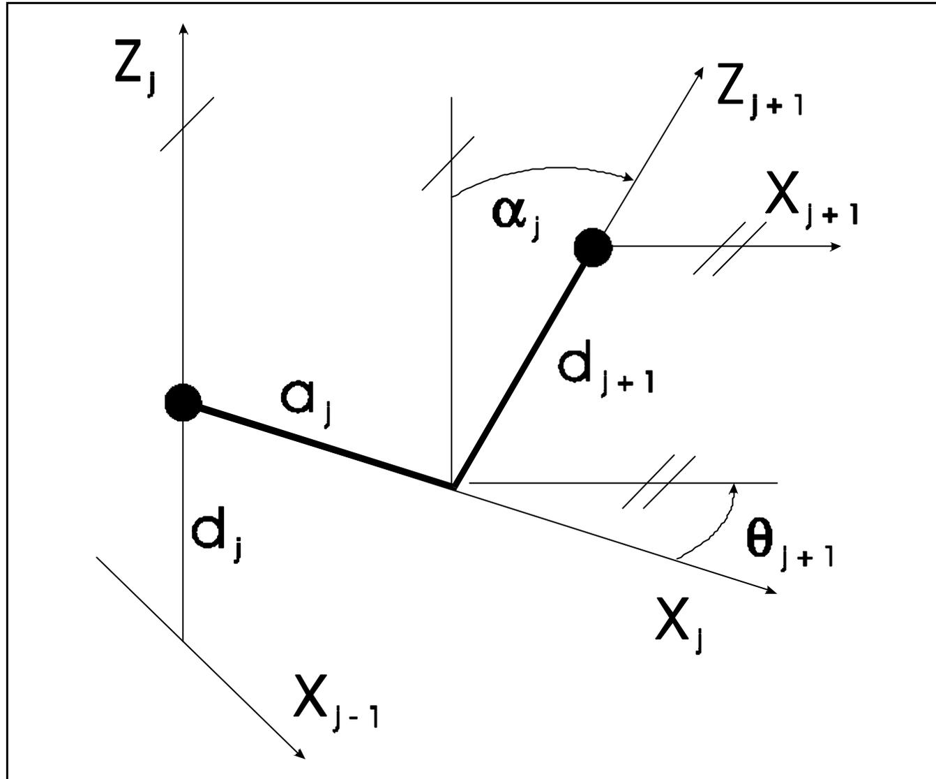
Fig.3.6: A kinematic scheme for manipulator link parameters according to the H-D notation.
