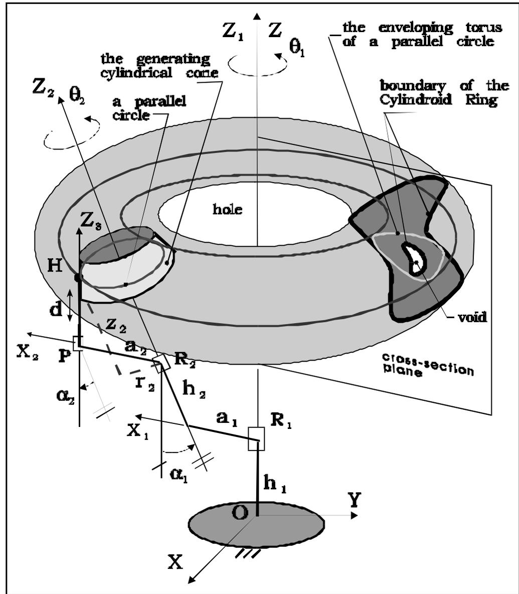
Fig.3.12: Design parameters and topology in the generation of so-called Cylindroid Ring workspace for
