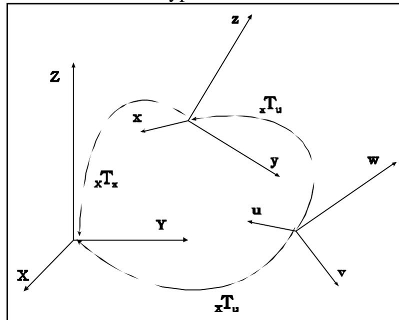
Fig.3.8: A scheme for indicating which frames a transformation matrix is formulated with respect to.
