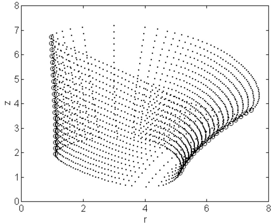
Fig.2. Cross-section of a Cylindroid Ring workspace volume computed as an union of generating tori for a telescopic RRP manipulator with  $a_1 = 3$  u,  $a_2 = 2$  u,  $d_1 = 0$  u,  $d_2 = 1$  u,  $\alpha_1 = 30$  deg,  $\alpha_2 = 30$  deg.,  $d_{\min} = 1$  u,  $d_{\max} = 6$  u, ( u is a unit length).
