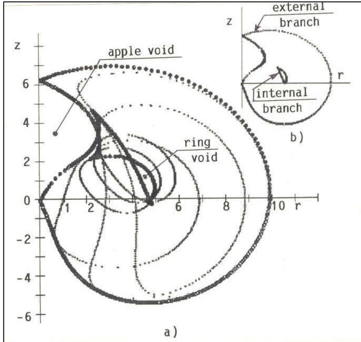
Fig.3.13: Workspace cross-section of a 4R manipulator with  $a_1 = 3 u$ ,  $a_2 = 4 u$ ,  $a_3 = 2 u$ ,  $a_4 = 5 u$ ,  $\alpha_1 = \alpha_2 = \alpha_3 = 60 \text{ deg}$ ,  $d_2 = d_3 = d_4 = 1 u$ . ( $u$  is the unit length)
