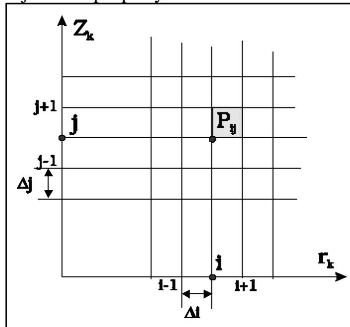
*Fig.3.14: A grid of scanning process for binary mapping of workspace cross-section.*
