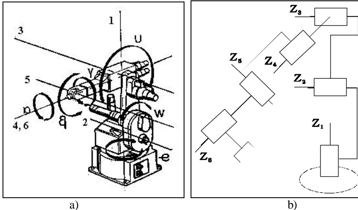
*Fig.3.5: An example of modeling an industrial robot: a) the mechanical design; b) the corresponding kinematic functional scheme.*
