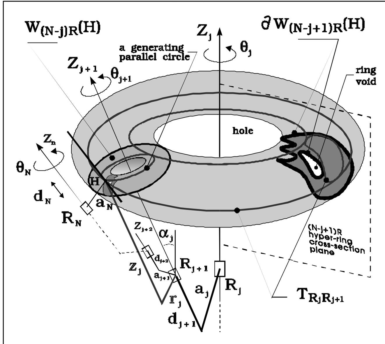
Fig.3.11: A descriptive view of workspace generation for serial manipulators with revolute joints.
