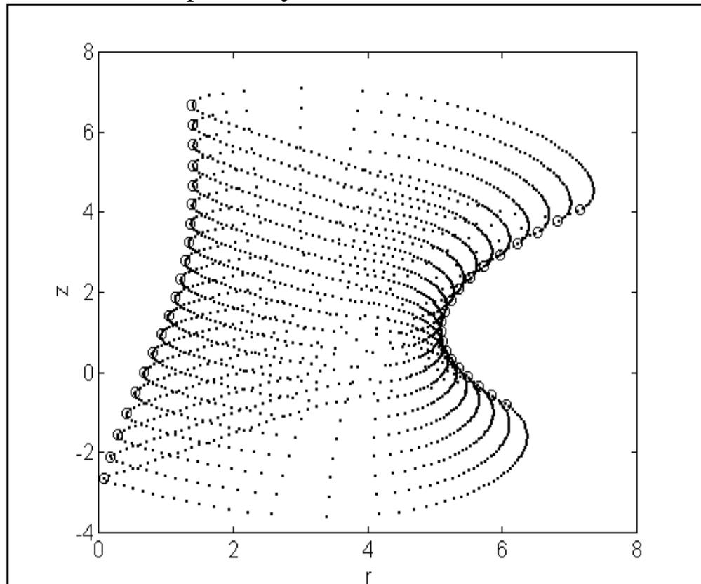
Figure 3.17: Cross-section of a workspace boundary computed as tori envelope segments (circle points) and toroidal covers (dotted points) for a telescopic manipulator arm with  $a_1 = 3 u$ ,  $a_2 = 2 u$ ,  $h_1 = 0 u$ ,  $h_2 = 2 u$ ,  $\mathbf{a}_1 = 30 \text{ deg}$ ,  $\mathbf{a}_2 = 30 \text{ deg}$ .,  $d_{\min} = -5 u$ ,  $d_{\max} = 5 u$ , ( $u$  is a unit length).
