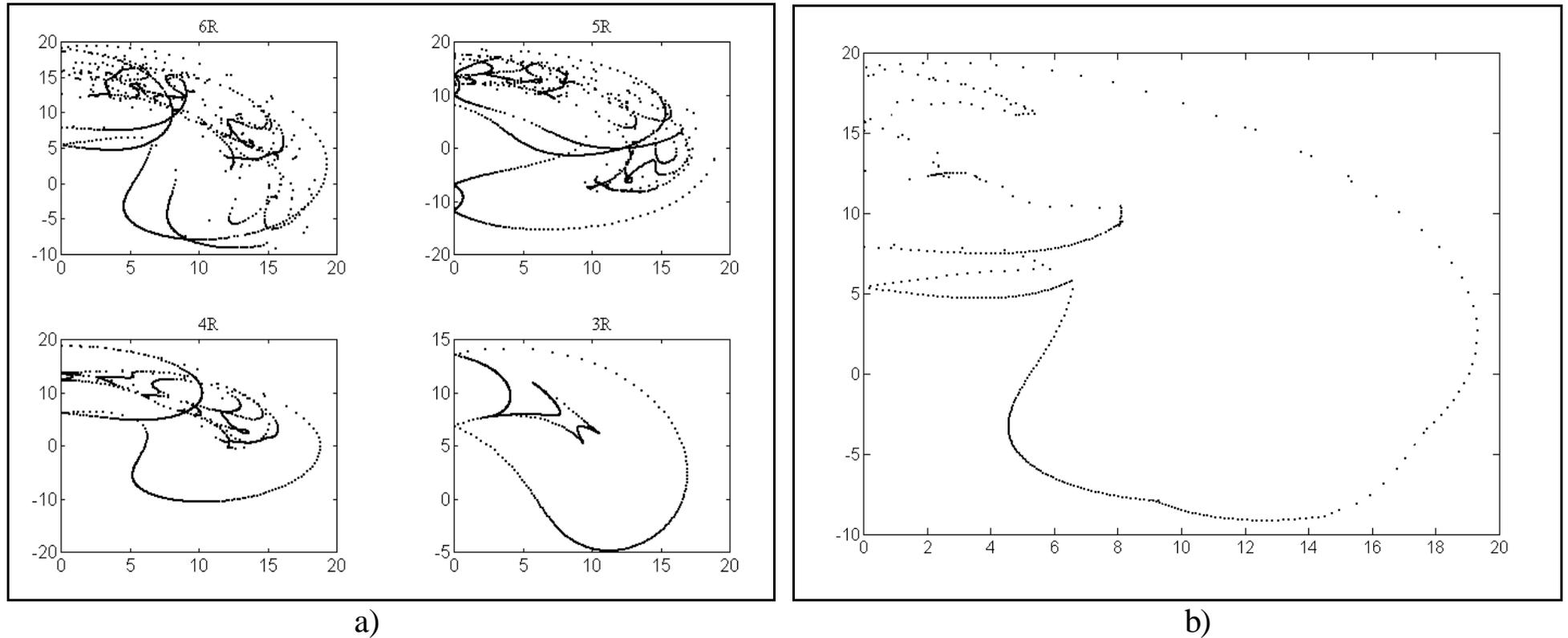
*Fig.3.16: Workspace cross-sections of a 6R manipulator with  $a_i = i u$  ( $i = 1, \dots, 6$ ),  $d_1 = 0 u$ ,  $d_i = (i-1) u$  ( $i = 2, \dots, 5$ ), and  $\alpha_i = \pi/4$  ( $i = 1, \dots, 5$ ). ( $u$  is the unit length): a) the envelope boundary in the generating workspaces; b) the cross-section of primary workspace.*
