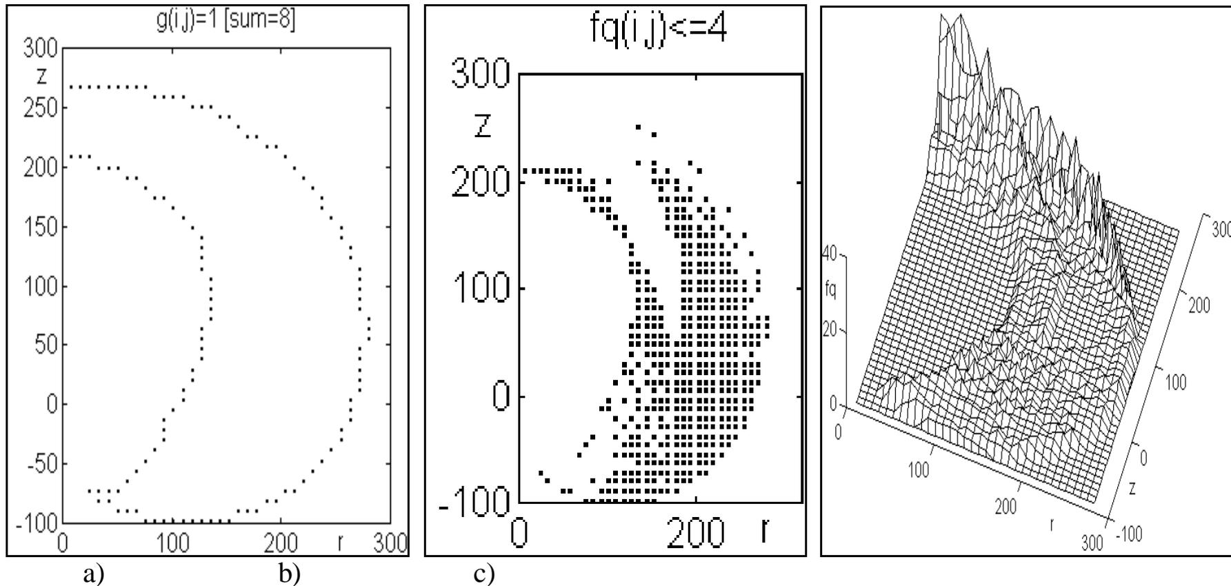
*Fig.3.15: Results of the binary matrix formulation for workspace evaluation of a robot manipulator COMAU SMART 6.100A with  $a_1 = 300$  mm,  $\mathbf{a}_1 = 90$  deg.,  $a_2 = 1,100$  mm,  $\mathbf{a}_2 = \mathbf{a}_3 = 0$  deg.,  $a_3 = 1,625$  mm, and  $b_1 = b_2 = b_3 = 0$ : a) cross-section workspace contour generated with sum = 8; b) cross-section area of secondary workspace with  $f_q(i,j) \leq 4$ ; c) a map for the frequency matrix  $f_q(i,j)$ .*
