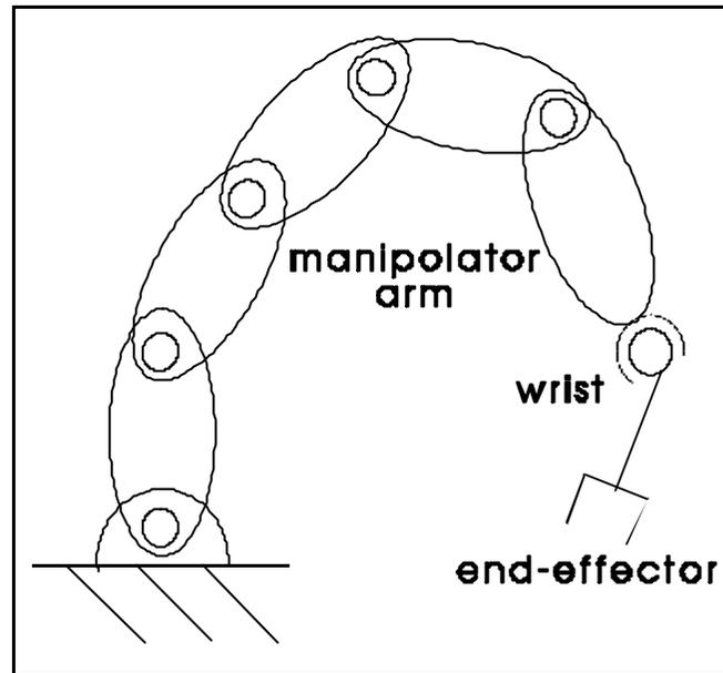
*Fig.3.1: A scheme for the manipulator architecture of a robot with the arm, wrist, and end-effector.*
